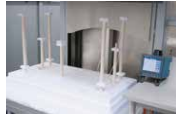
Measurement set-up in a high-temperature furnace
