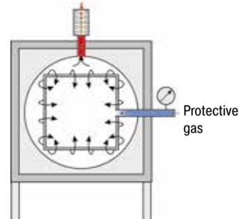
**Safety Concept for Heat Treatment under Flammable Process Gases**
